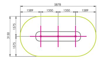
Clear Space Required (25mm tolerance added in each direction)
